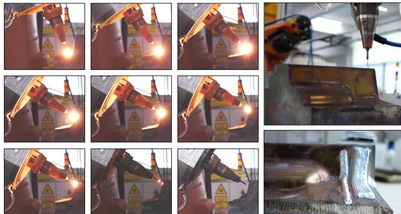
Fig. 2 AC-LMWD repair processing for irregular surface stamping molds
