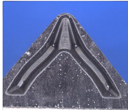
Fig. 1 Laser milling of PCD chip-breaking groove after path optimization
